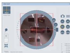
Left: Picture of the specimen captured by the camera equipped inside the chamber. Right: Camera image transferred to the SEM MAP screen for navigation.
