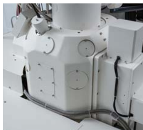
left: external view of the specimen chamber featuring 18 accessories ports
